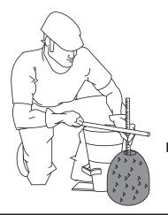
Figure 35-F. Slump Test (Measurement)
